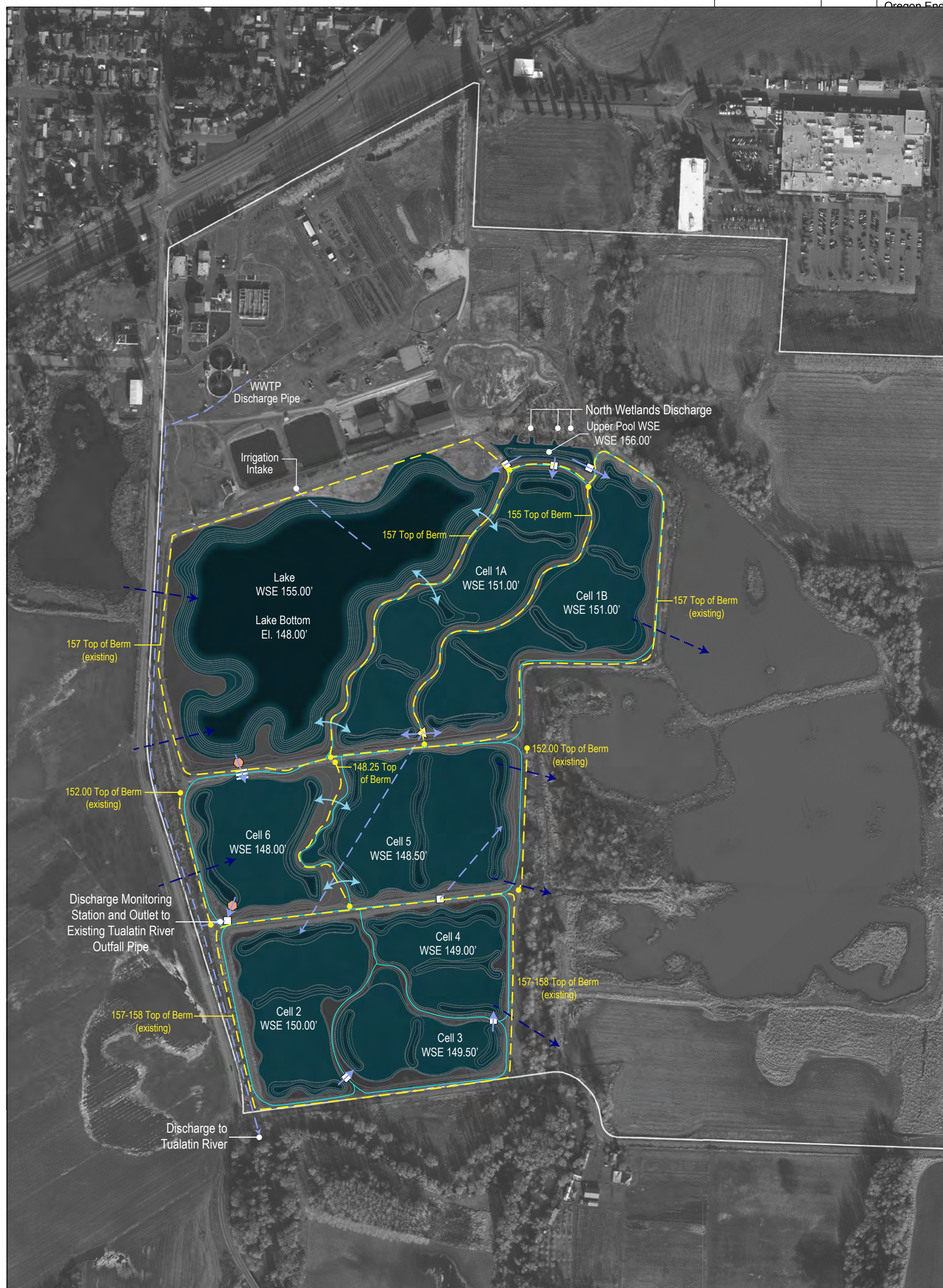
Figure 5-2 Basis of Design Normal Operating Water Level South Wetlands Forest Grove, OR
